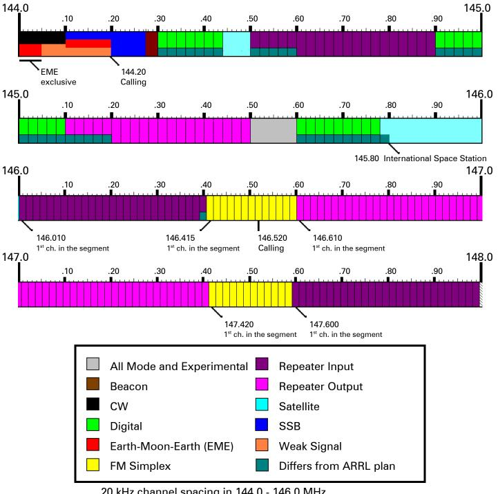
20 kHz channel spacing in 144.0 - 146.0 MHz 15 kHz channel spacing in 146.0 - 148.0 MHz In the ARRL plan all channels are 20 kHz.
